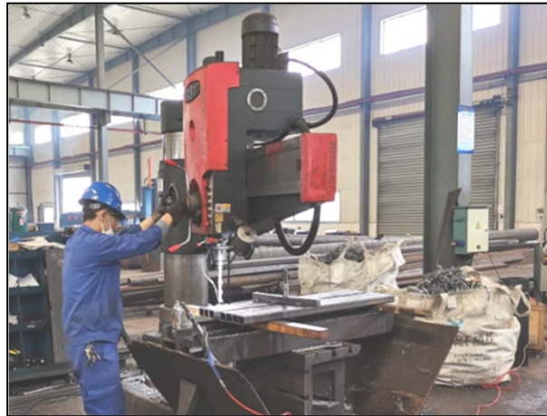
Radial Drill (Ø60mm)
