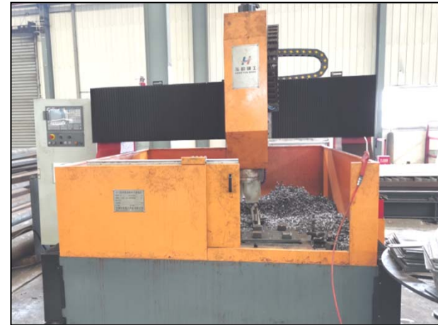
CNC Drill (Ø40mm)
